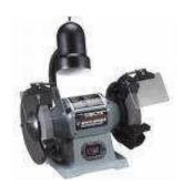
• If a pedestal or bench grinder fails the pre-use inspection, notify your supervisor and remove the grinder from service by attaching a red tag that states "OUT OF SERVICE." Complete red tag with appropriate information.
